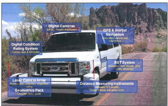
Laser Camera Array (LCA)
